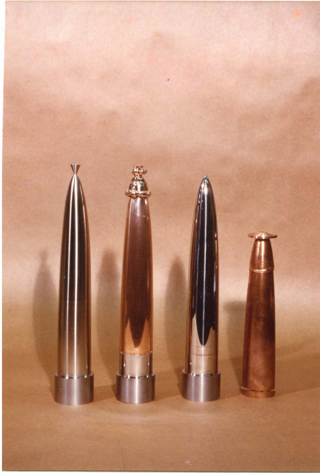
Plate B.I: Steps in manufacture of compound parabolic concentrators. Left to right: unpolished stainless steel mandrel, mandrel after electroforming concentrator, polished mandrel after removal of concentrator, and the finished concentrator.
